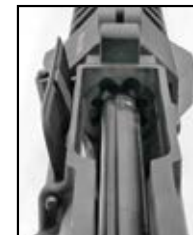
Insert scraper into star chamber and twist to scrape
