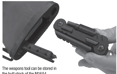
Use small brush for light debris removal. Tool can be removed and replaced with other Otis components.
