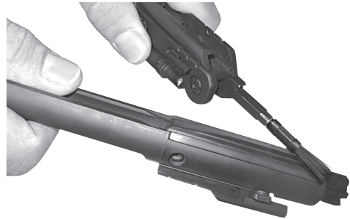
Use small brush for light debris removal. Tool can be removed and replaced with other Otis components.
