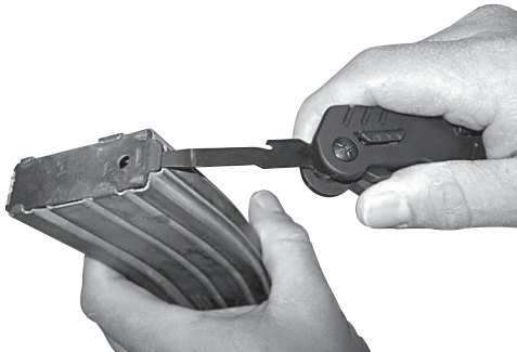
Flat head driver can be used for screws or adjustments. Pictured is the base plate of a magazine being removed.
