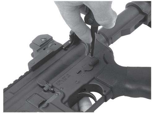
Punch can be used on pins on receiver.
