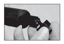
Assemble scraper and nose on tool.
