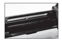
Turn clockwise to scrape fouling in the star chamber area.
