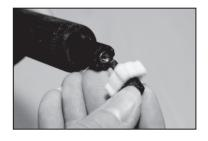
Replace scraper with cleaning pad and insert in chamber.
