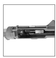
3. Remove charging handle and tool from upper receiver.
