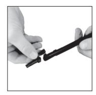
2. Insert charging handle with attached tool back in normal position in upper receiver. When fully seated, tool will clean out vent hole area.
