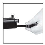
4. Rotate tool 90 degrees to unlock from charging handle.
